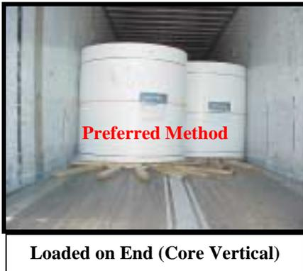
Rolled paper can be loaded using various methods but the preferred method from a safety standpoint is loading rolled paper on end with the core vertical to the floor. (See photo at left.) Other variations, like the one loaded on bilge in the photo at right, cause load stability issues during transportation.
